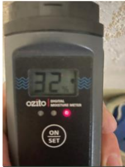
Moisture test of walls. Ranged from 30 to 50 % on some walls
